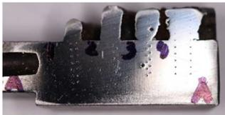
Fig. 4: Points at which hardness was measured.
