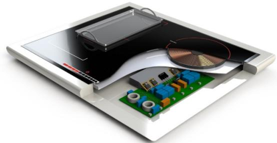
Fig. 1. Typical induction cooktop with flexible surfaces.
