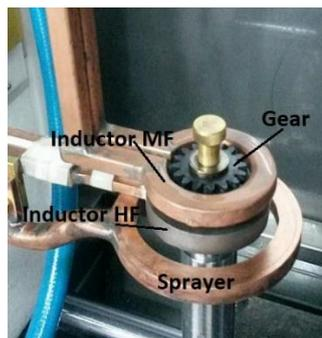
Fig.3 Configuration of the inductors-sprayer system during CDFIH process [11]
