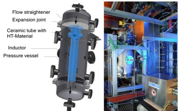
Fig. 2. Component level: CAD-model (left) and experimental setup (right) of the air heater unit based on induction heating of packed bed
